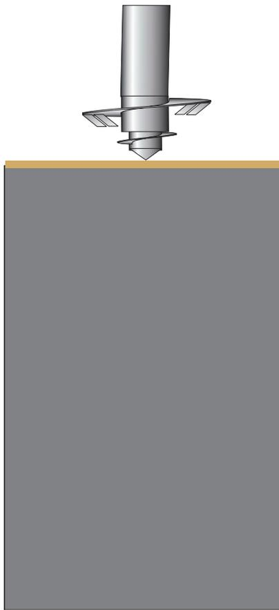
Positioning of the tooling. The mixing tool is mounted on a high revolutions ABI auger drive while the suspension supply is hooked up. (suspension= water cement mixture in various ratios)
