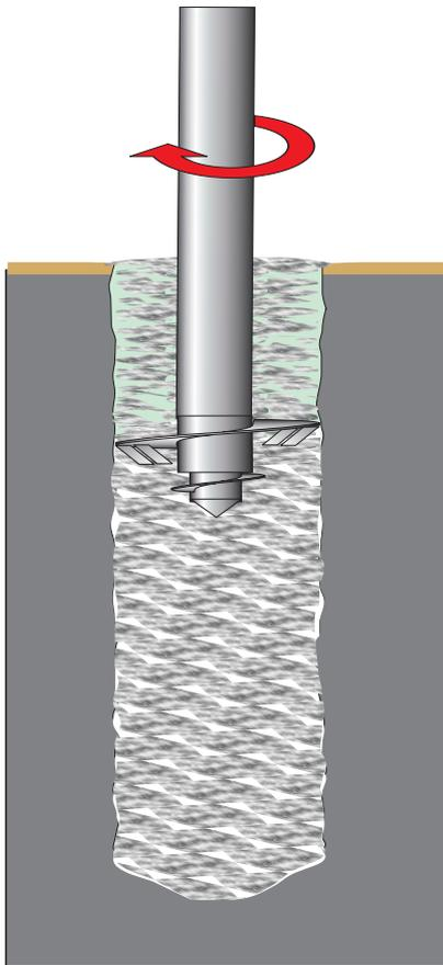
The developed mixture from soil and suspension gets mixed again during withdrawal and suspension is continuously pumped.
