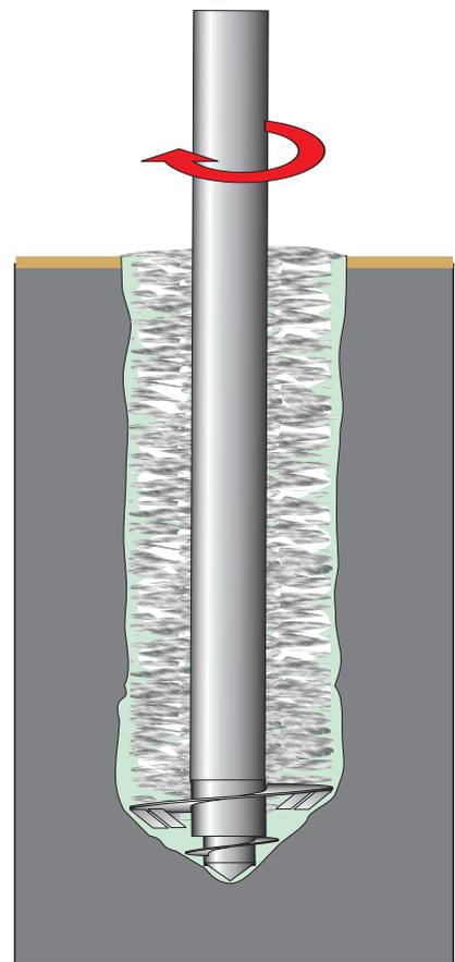
Suspension is constantly pumped to the mixing tool while lowering to the required depth.
