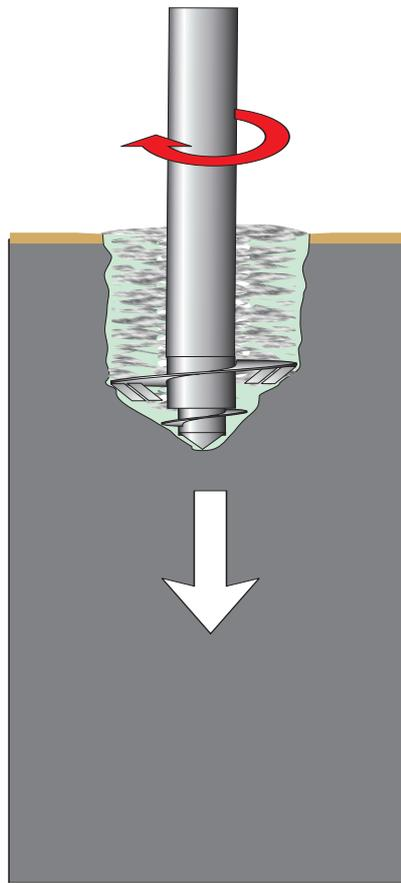
Lowering the mixing tool into the soil with 100 – 200 rpm. A substantial amount of soil gets mixed with under pressure injected suspension.
