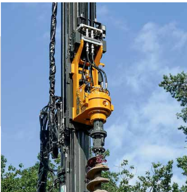
The auger drive MDBA can be used for several applications: e. g. for pre-drilling, CFA drilling as well as for soil mixing.
