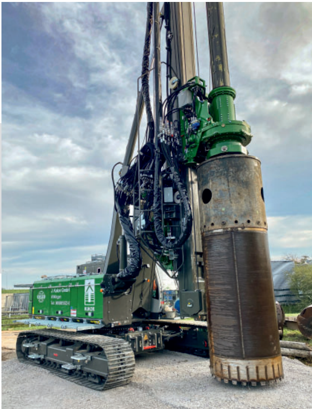
The telescopic undercarriage is equipped with mechanical connections for a casing oscillator (with an integrated control unit) for assisting in inserting large diameter casings in difficult soil conditions.
