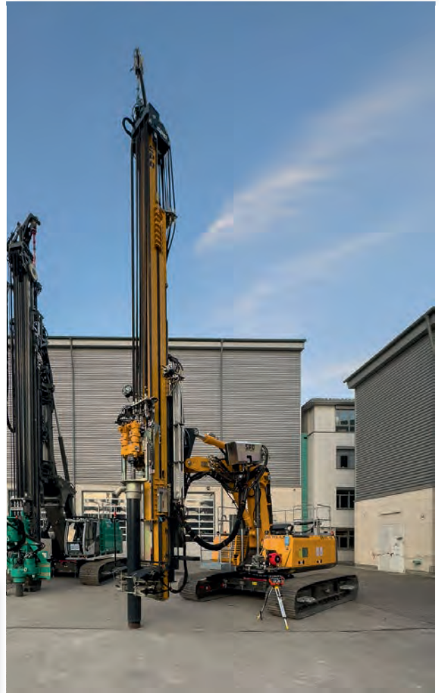
A visit from Sweden. The subsidiary SPD from Sala presented its T13 with a down-the-hole hammer and remote control.
