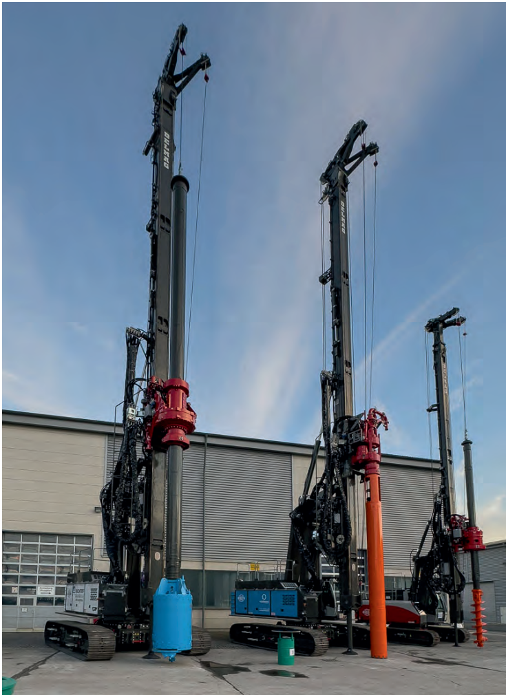
DELMAG drill rigs. From large to small: RH 38 with rotary head and a box-type drill, RH 34 with VDW equipment and the compact model RH 14 with Kelly drilling equipment.
